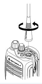
Turn the antenna counterclockwise to remove it.
