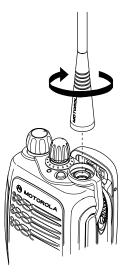
Turn the antenna clockwise to attach it.
